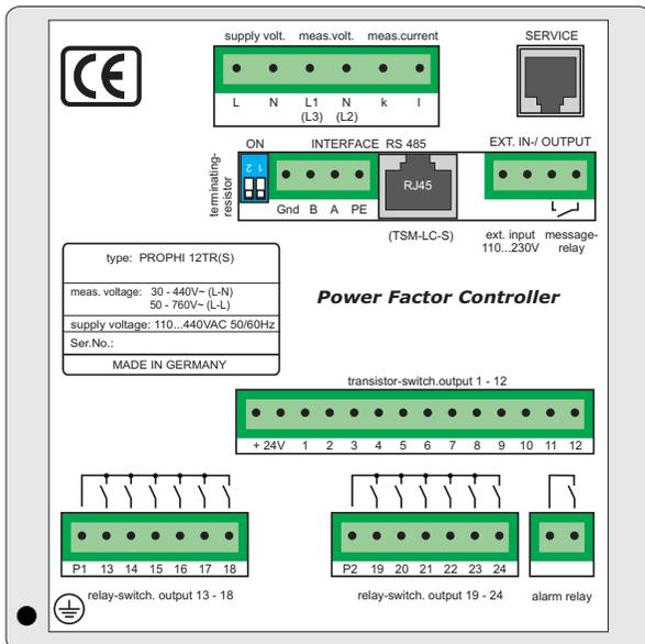
**Section 2 Installation and connection of the controller**
