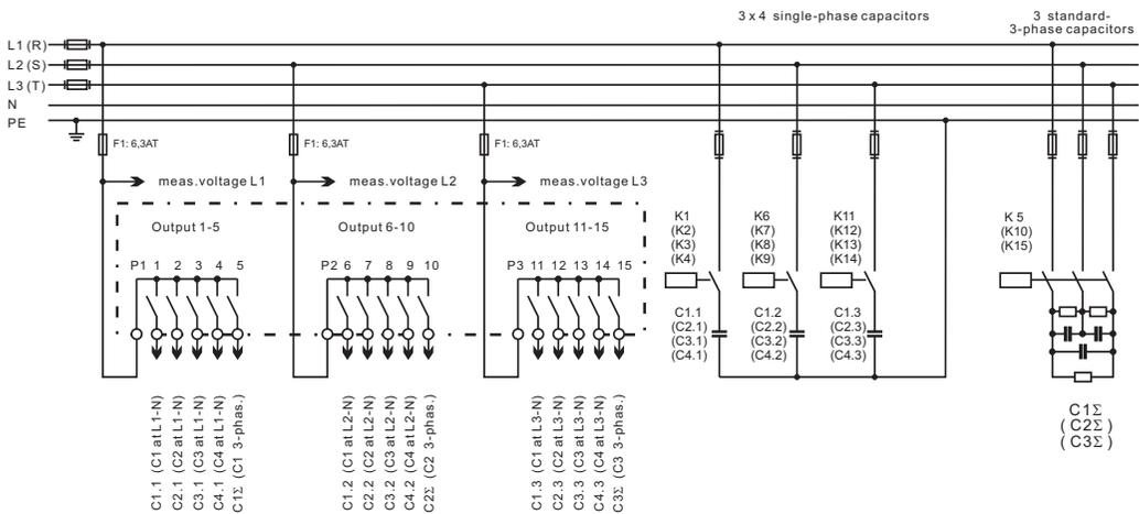
In case of the setting the controller will automatically assign the capacitors according to the wiring diagram.
