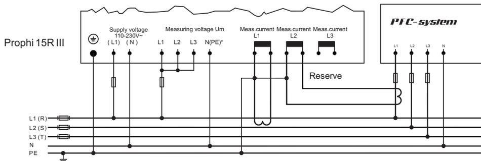
**Connection of current transformer / sum current transformer**
