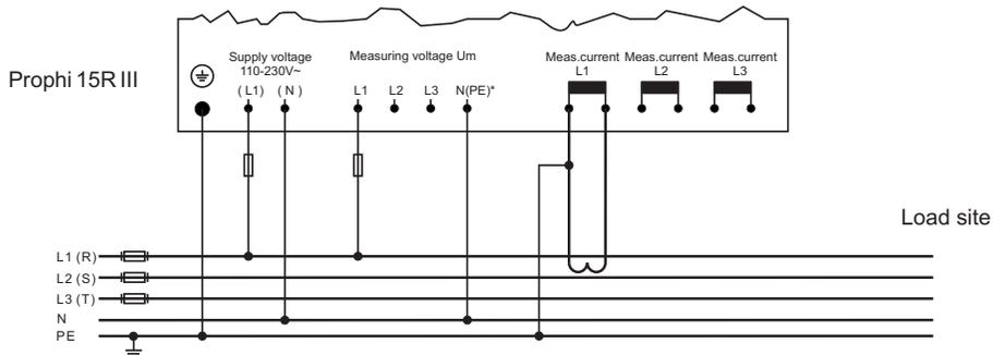
Alternative 3: single-phase measuring as alternative 2, but with capacitor current measuring in the compensation system for collection of real capacitor currents.
