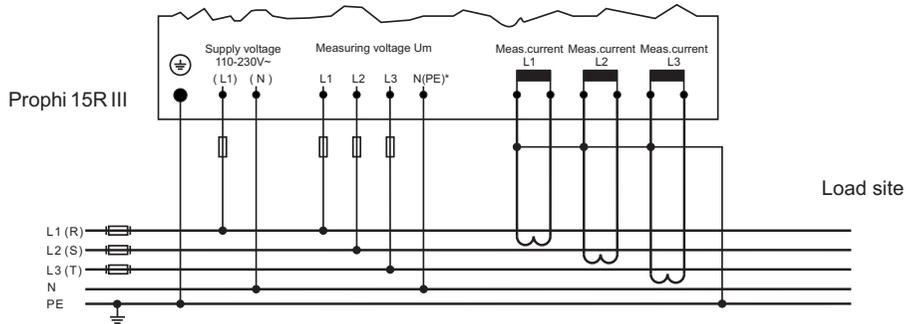
Alternative 2: single-phase measuring via current transformer in L1 Values extrapolated (balance assumed).
