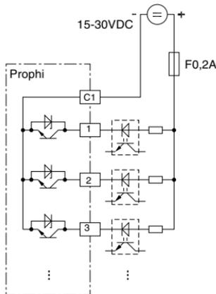
Diagr.: Connection example "Transistor outputs"
