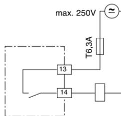
Diagr.: Connection diagram alarm output
