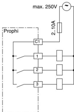
Diagr.: Connection example "Relay outputs"
