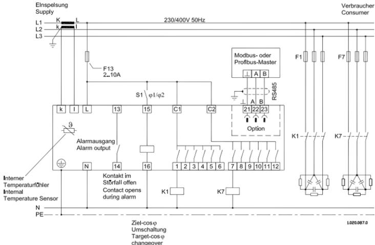
Diagr.: Connection example, power factor controller with measurement and supply voltage L-N, 12 relays outputs, target cos(φ) changeover and alarm output.
