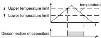
Diagr.: Overtemperature disconnection with hysteresis
