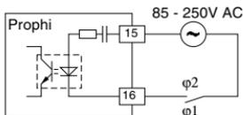
Diagr.: Connection diagram target-cos(phi) changeover
