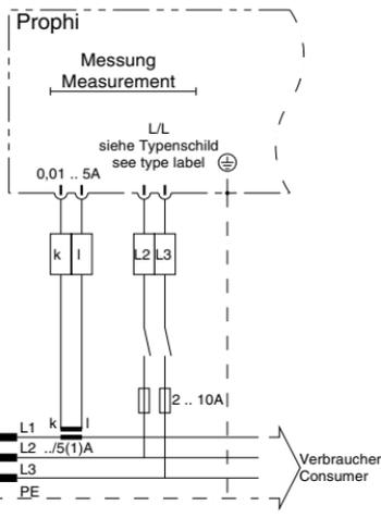
Diagr.: Connection of measurement and supply voltage (L2-L3) and current transformer.
