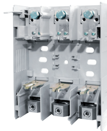
RBK 1 pro VD-M for installation on mounting plate, picture of fuse switch disconnect without fuse links cover and terminal shrouds, top cable terminal - M screws, bottom cable terminal - V-clamps, (RBK 1 pro VG-M - bottom cable terminal - M screws, top cable terminal - V-clamps)
